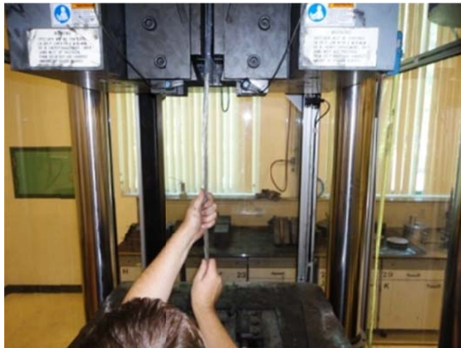
Figure 4.9 Sample carefully placed in jaws to prevent inadvertent grit removal.
