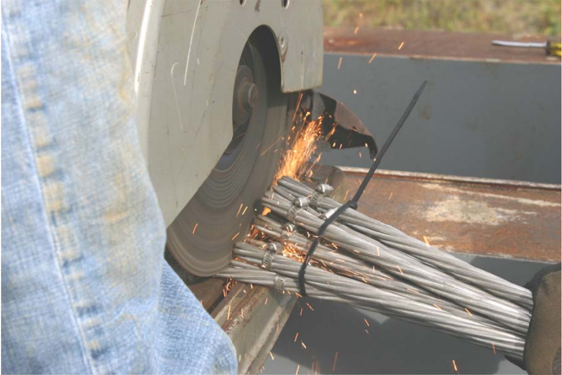
Figure 5.4 All twelve hose clamp-restrained strands cut to length.
