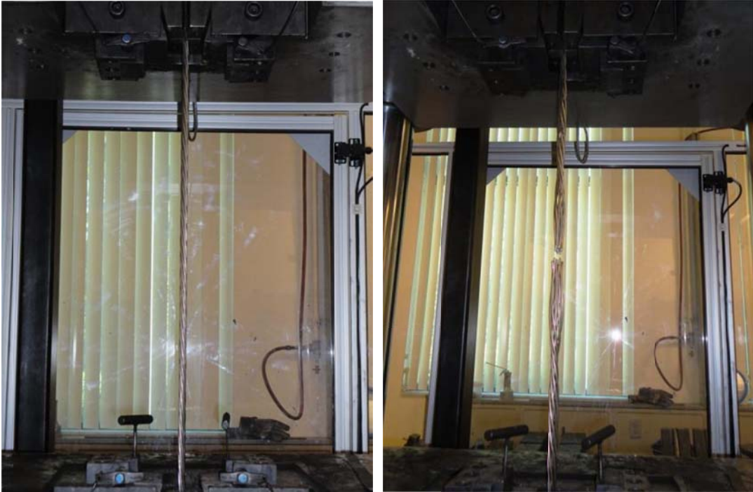
Figure 4.11 Testing after extensometer removal (left); after failure (right).
