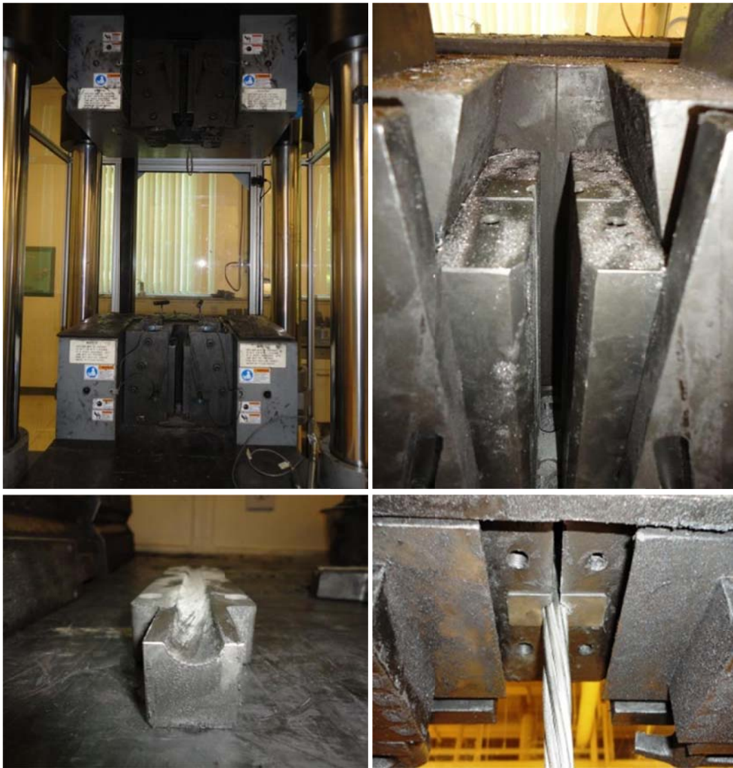
Figure 4.5 Universal Testing System (top left); testing jaws (top rt); tapered ½in half-round insert (bot left); strand in jaws (bot rt).
