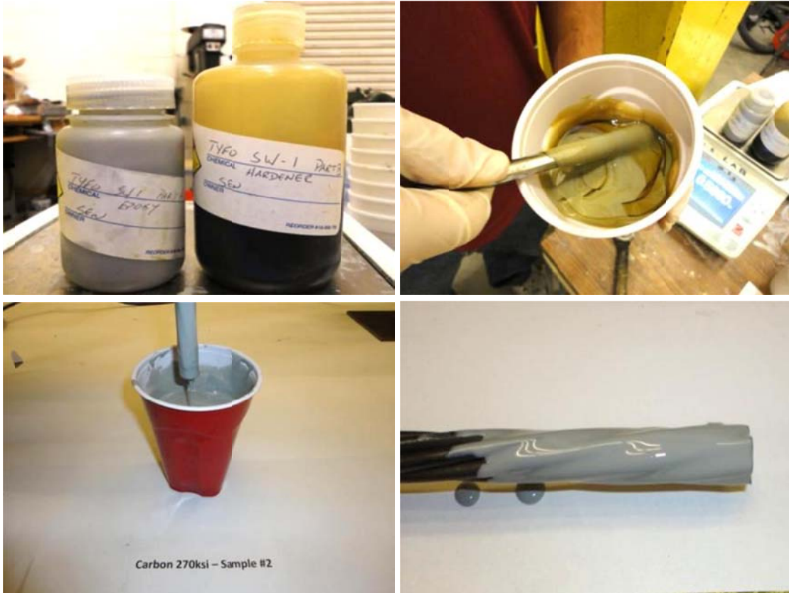
Figure 4.3 Tyfo SW-1 epoxy (top left); mixing two-part epoxy (top rt); strand dipped in epoxy (bot left); epoxy coated strand end (bot rt).
