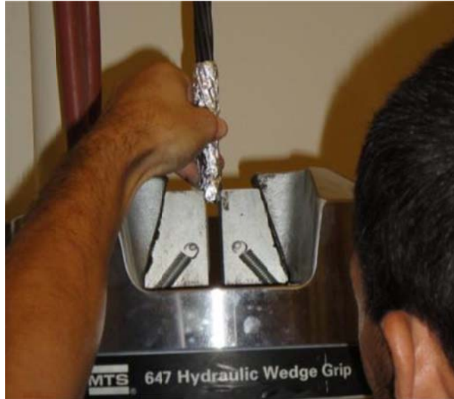
Figure 4.1 Placement of foil covered strand in testing jaws.
