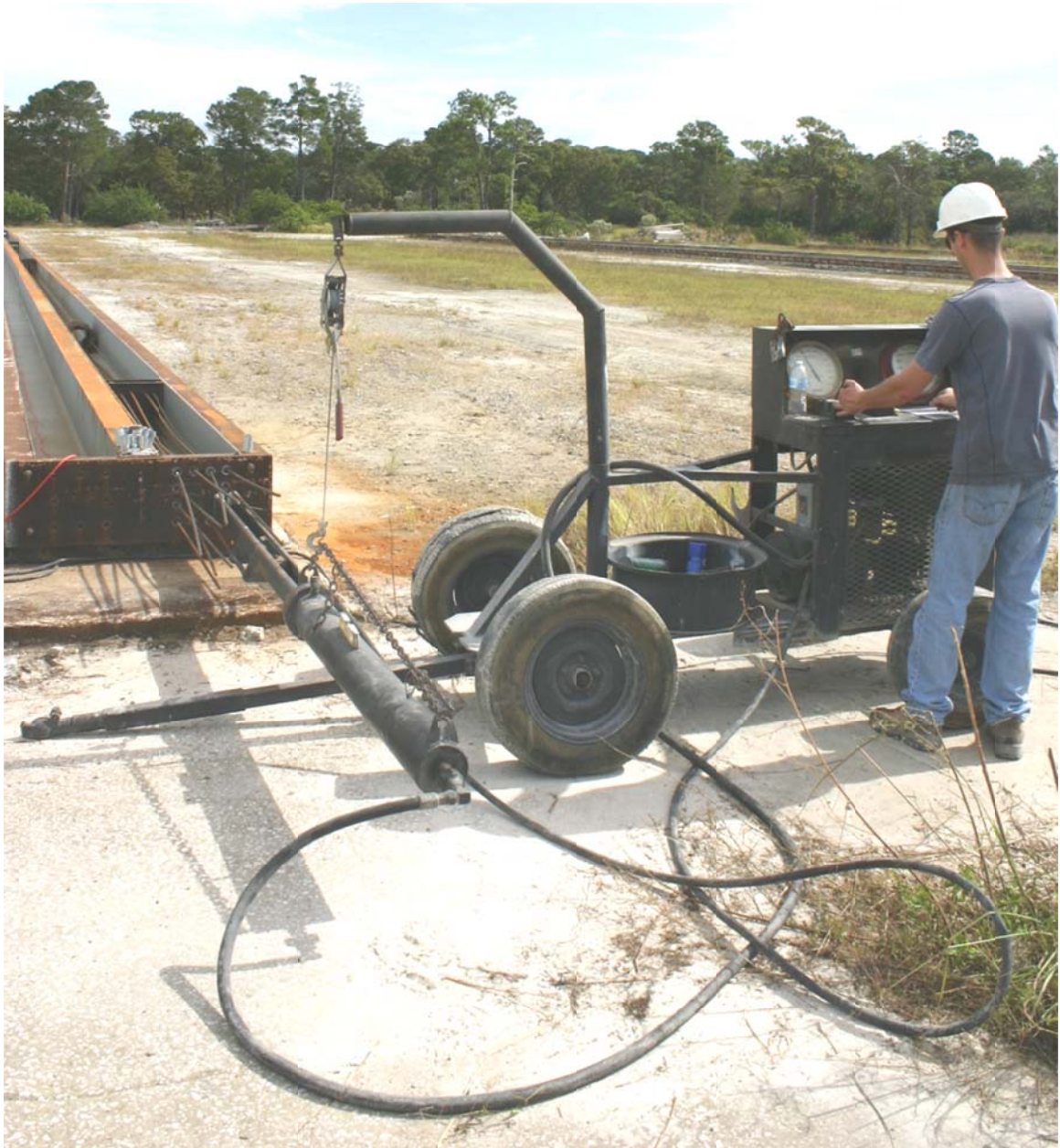
Figure 5.13 48in stroke hydraulic jack used to cycle and bring strands to design load.
